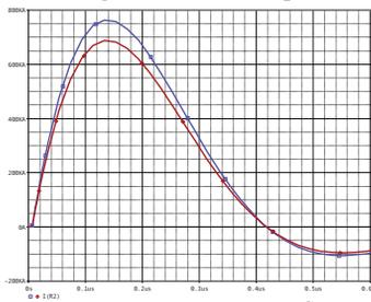
Figure 5: Simulated waveform of the stage with 20 brick and 80nF capacitor in match load (not consider loss).
