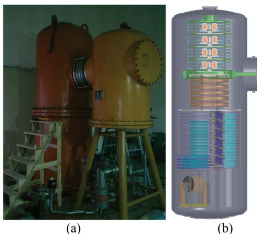
Figure 4: The 800 kV/30 mA electron accelerator and its power supply structure. (a) The accelerator. (b) The profiles of the power supply.
