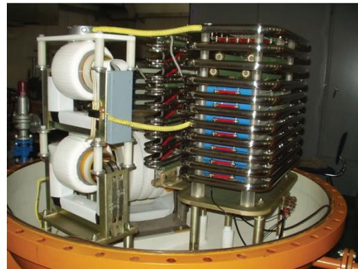
Figure 2: The 300 kV/60 mA power supply for electron curtain accelerator in Suzhou.
