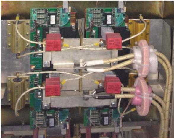
Figure 4: Converter's H-bridge.
