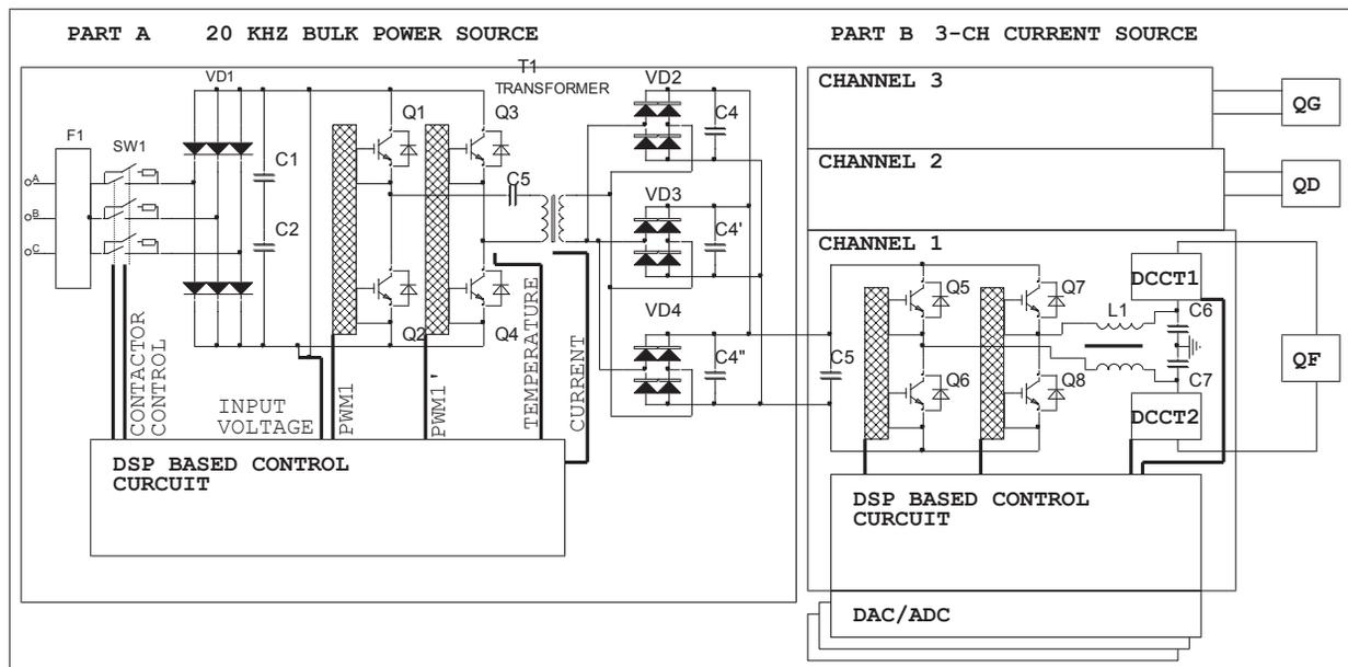
Figure3: 3-channel current source circuit diagram.
