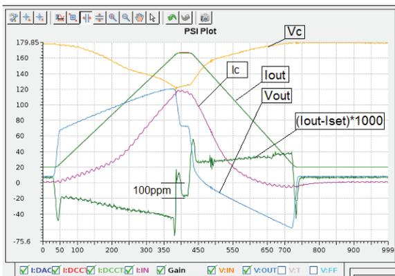
Figure 4: 1Hz 170A ramp QF source waveforms.
