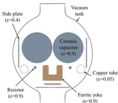
Figure 2: Slice through cross-section of an MKI magnet.
