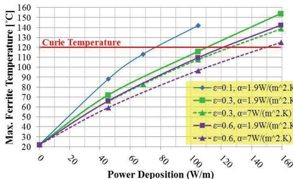
Figure 4: Predicted max. ferrite temperature versus total power deposition per m length of ferrite yoke, for various emissivities of the inside of the tank and convection ( $\alpha$ ).
