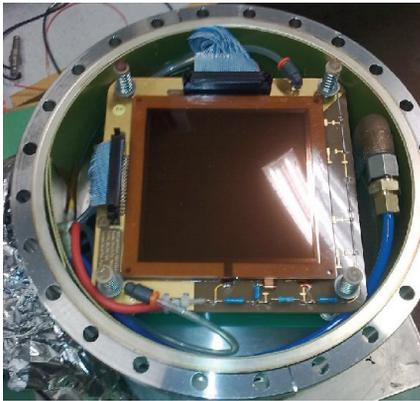
Figure 2: Single-GEM device installed inside the pendulum.
