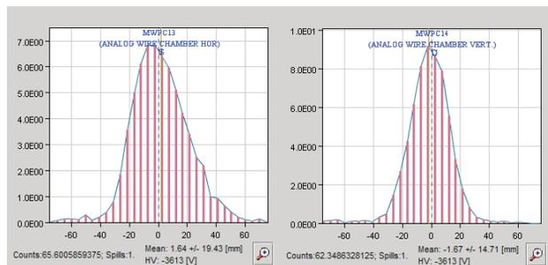
Figure 4: First profile readouts from the ‘big’ prototype GEM (200x200mm) on December 2nd 2012.
