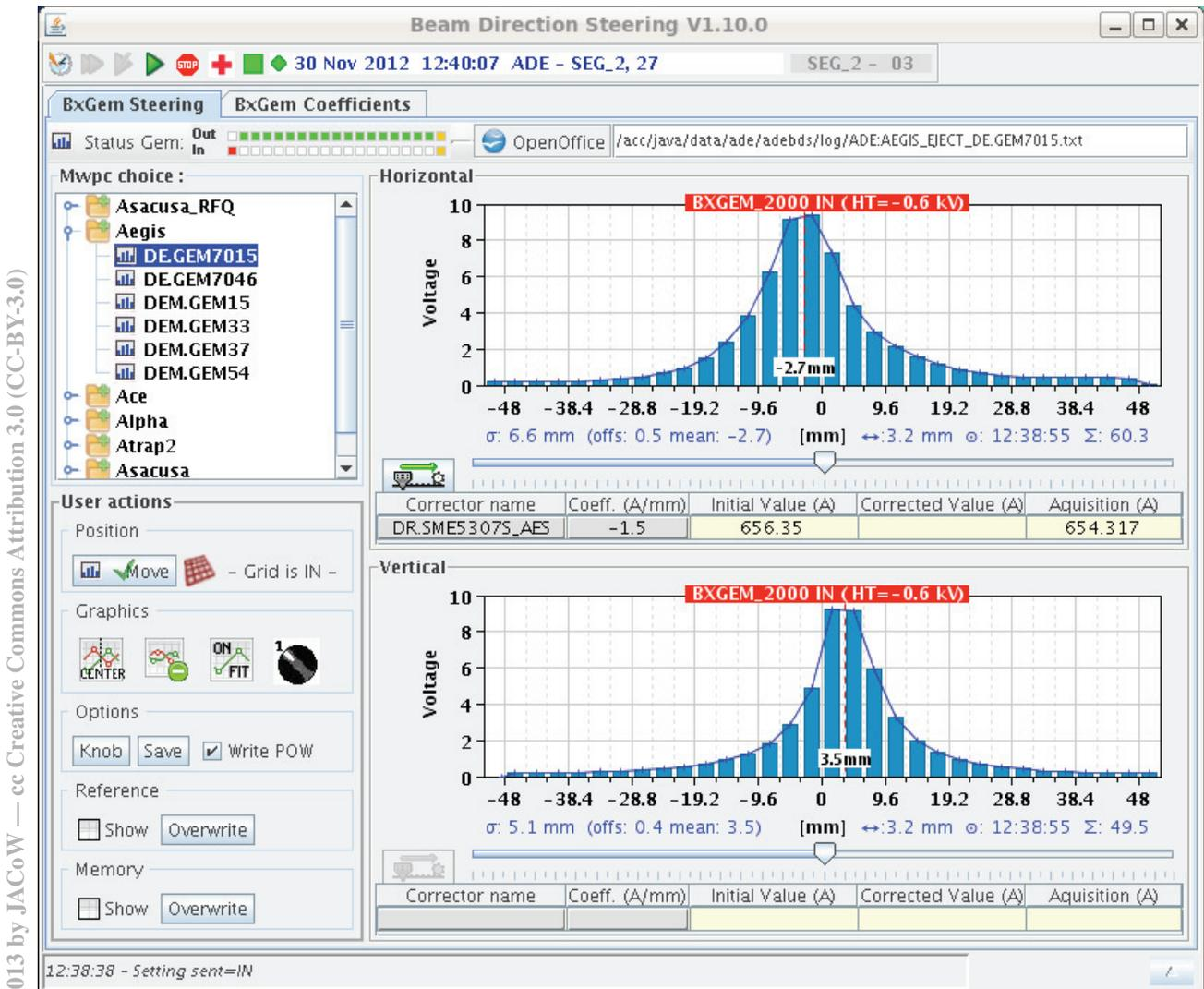
Figure 3: Simultaneous horizontal and vertical readout from a single-GEM detector using the new acquisition system. The 32 channel profiles are here acquired with 3.2 mm resolution. 1.6 mm pitch is also an option.
