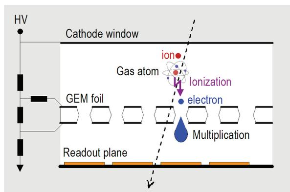
Figure 1: GEM detector principle.
