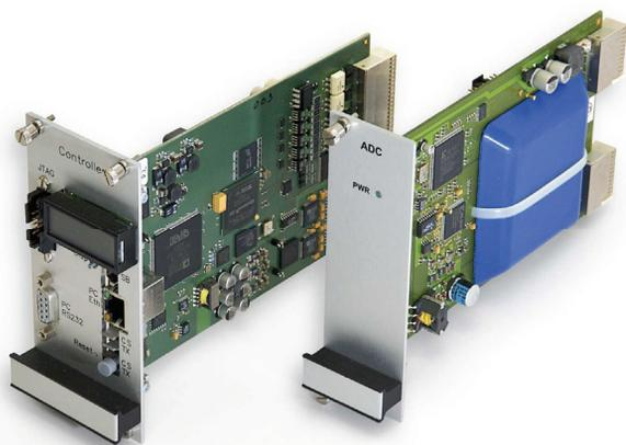
Figure 3: Controller board and high-stability ADC.
