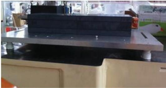
Figure 6: Increasing the distance between backplane and ground.
