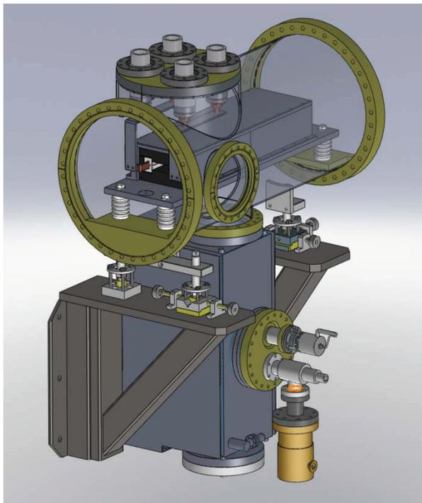
Figure 2: TPS booster injection kicker. (including all the components in the vacuum chamber and girders).
