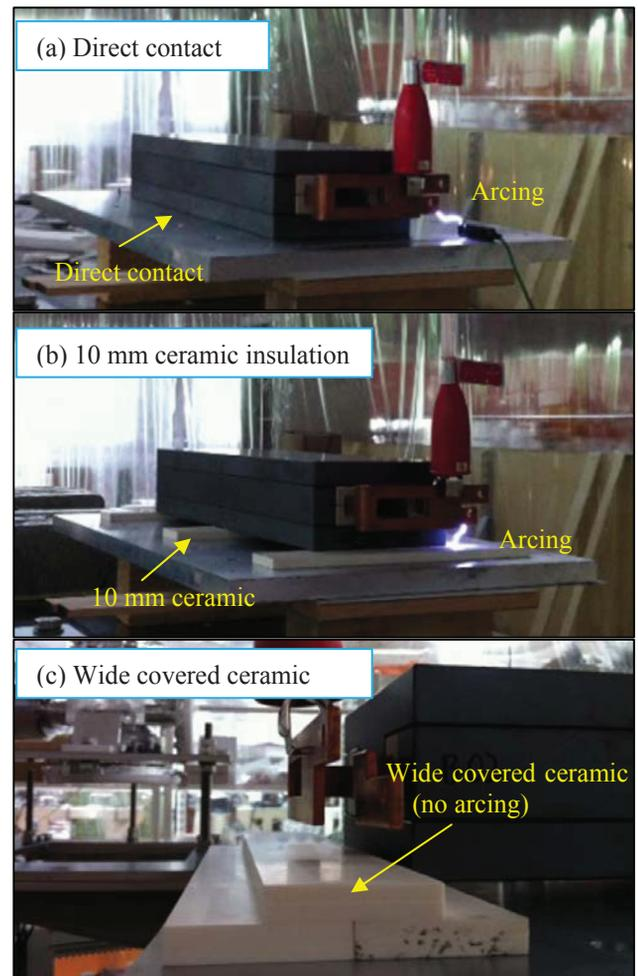
Figure 3: The experimental setup for DC withstand voltage test.
