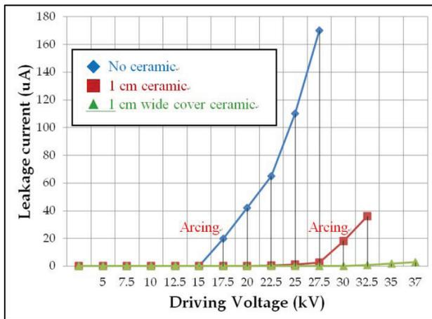
Figure 4: The HV test results.
