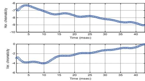
Figure 9: Measured uncompensated chromaticity.
