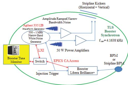
Figure 5: Functional block diagram of the new tune monitor for TLS booster.
