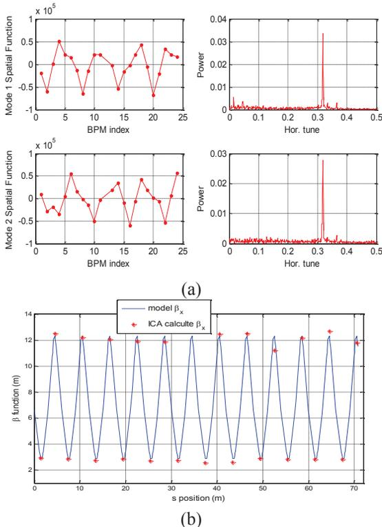
Figure 4: Preliminary results to apply ICA to calculate horizontal beta function using BPM turn-by-turn data. (a) Mode 1 and mode 2 spatial and temporal functions. (b) Beta Function.
