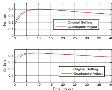
Figure 8: Quadrupole adjustment to avoid vertical 1/3 fractional tune resonant.
