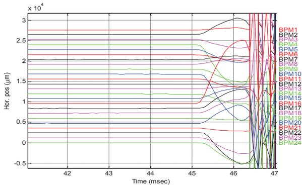
Figure 2: Horizontal beam position variation during beam extraction bumper magnets triggered.
