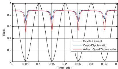
Figure 7: Tracking errors among quadrupole and dipole.
