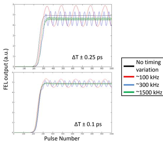
Figure 4: FELO simulation of the effect of small timing variations of 0.5ps and 0.2ps on the FEL output.
