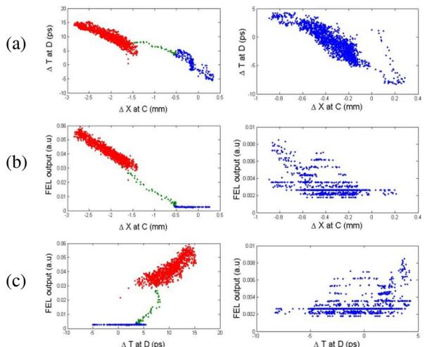
Figure 3: Correlations between BAM, BPM and FEL measurements for each bunch with (left) and without lasing (right).
