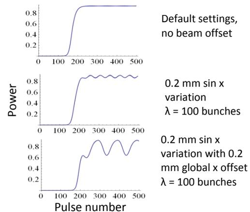
Figure 5: GENESIS simulation of the effect of small positional displacements on FEL output.
