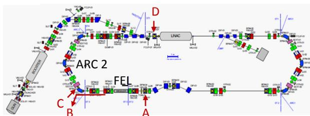
Figure 1: Layout of the ALICE accelerator and beam monitoring positions.
