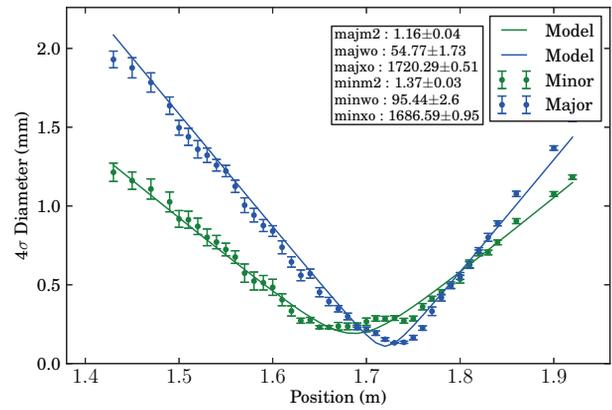
Figure 2: Measured laser propagation in both axes.
