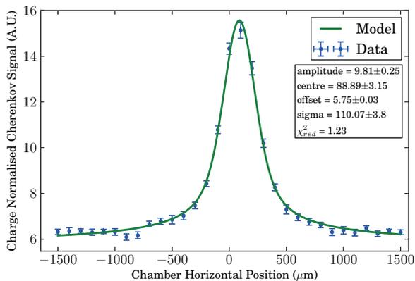
Figure 4: Horizontal scan of the electron beam.
