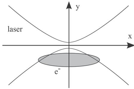
Figure 1: Schematic of laser propagation across a large aspect ratio electron beam (not to scale).
