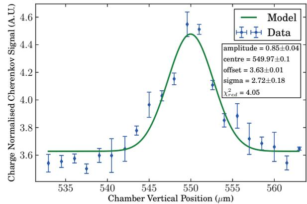
Figure 3: Initial vertical scan of the electron beam.
