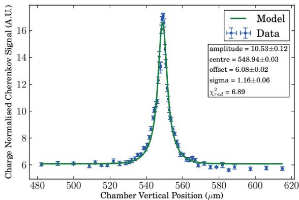
Figure 5: Detailed nonlinear vertical scan of the electron beam.
