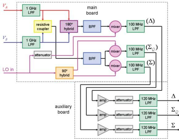
Figure 2: FONT analogue signal processor design.
