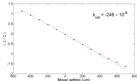
Figure 5: Example BPM calibration illustrating the dynamic range of the processor, showing  $\Delta/\Sigma$  for each mover setting (blue) and linear fit to data (red). The calibration is obtained for the linear region where  $|\Delta/\Sigma| < 1$ .
