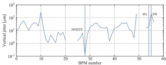
Figure 6: Vertical beam position RMS for the BPMs on the ATF2.
