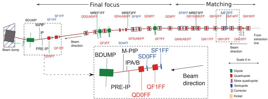
Figure 3: Layout of the ATF2 from the  $\beta$  matching section onwards to the IP and dump. The IP region is zoomed [5].
