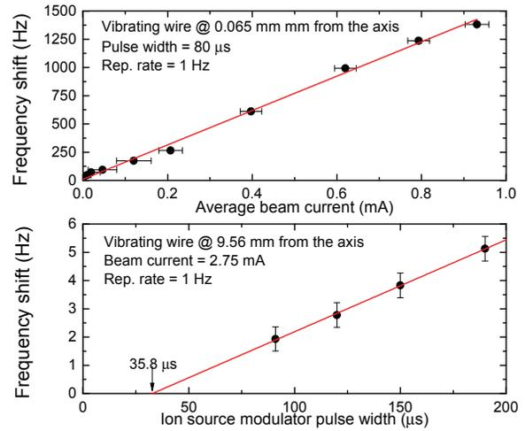
Figure 3: Linearity of the frequency shift of the LA-VWM with respect to the average beam current (top) and the ion source modulator pulse width (bottom).
