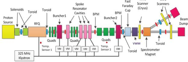
Figure 2: Block diagram of the HINS beamline configuration used for the beam test of the LA-VWM. The ambient temperature is monitored by the two temperature sensors shown in red circles.
