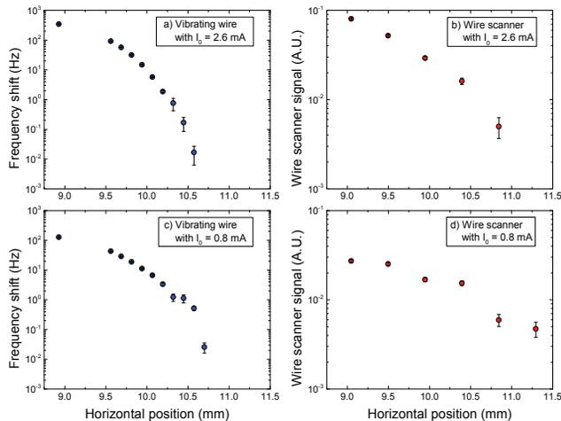
Figure 6: Comparison between the beam profile measurements in the tail region (i.e., around the horizontal position of 10 mm in Fig. 4): (a) LA-VWM for  $I_0 = 2.6$  mA, (b) wire scanner for  $I_0 = 2.6$  mA, (c) LA-VWM for  $I_0 = 0.8$  mA, and (d) wire scanner for  $I_0 = 0.8$  mA. The beam pulse width and repetition rate are  $80 \mu s$  and 1 Hz for all cases.
