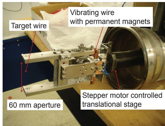
Figure 1: Picture of the large aperture vibrating wire monitor assembly.
