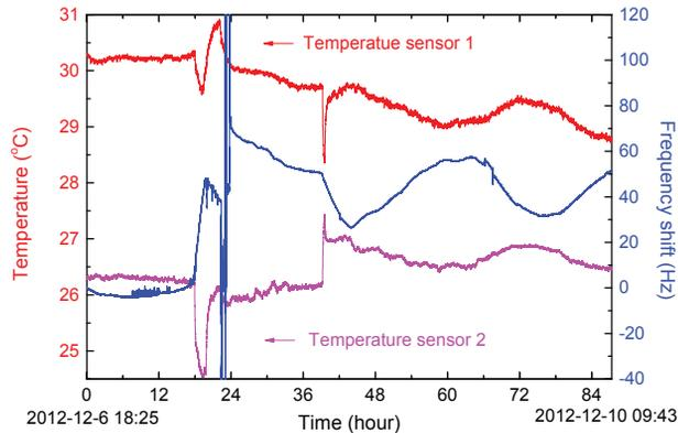
Figure 5: Effects of the ambient temperatures on the frequency change. A spike in the frequency at  $\sim 24$  hours after the start of the experiment occurred because we broke the vacuum of the beamline.
