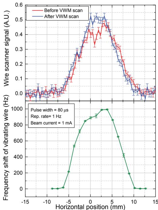
Figure 4: Comparison between the beam profile measurements with the wire scanner (top) and the LA-VWM (bottom). To obtain overall beam profile quickly, we use a coarse step size for the vibrating wire scanning. Also, a low beam current of  $I_0 = 1$  mA is used to enable frequency measurements at the beam core.
