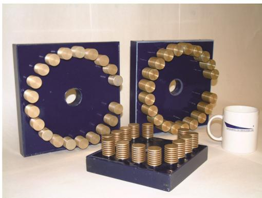
Figure 5: Three DTI 10 kV solid-state switchplates.
