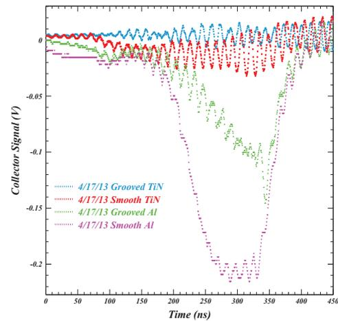
Figure 5: Comparisons of TR-RFA signals in the four vacuum chambers in the chicane for a 20-bunch train at 5.3 GeV, each bunch carrying  $1.28e11$  positrons, for the case of an ambient dipole magnetic field of 810 G.
