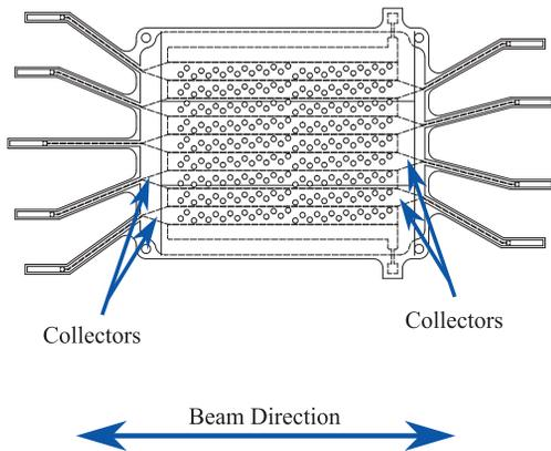
Figure 2: Bottom view of the nine collectors on the Kapton flex circuit. Cloud electrons migrate through the eighteen rows of 1.7-mm diameter holes during the buildup measurements.
