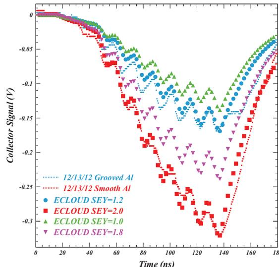
Figure 3: TR-RFA measurements and ECLLOUD model results for a 10-bunch train of 5.3 GeV positrons in the smooth and grooved uncoated vacuum chambers. The bunch spacing is 14 ns and the bunch population is 1.28e11. ECLLOUD models with peak SEY values of 2.0, 1.8, 1.2 and 1.0 are shown to illustrate the sensitivity of this comparison to the effective reduction in secondary emission afforded by the use of grooves as a mitigation technique.
