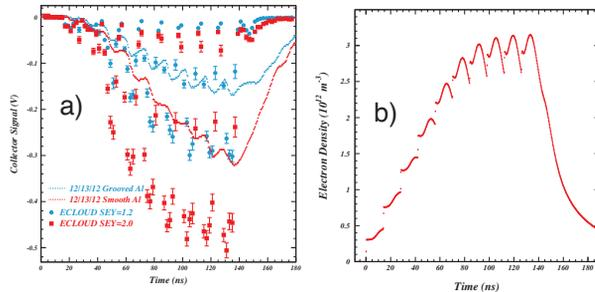
Figure 4: a) ECLLOUD model central collector signals for the smooth and grooved uncoated chambers as shown in Fig. 3, but with the TR-RFA time integration convolution removed in order to show the underlying time structure of the cloud signal. b) The modeled fluctuations in cloud density for the case of the 10-bunch positron train in the smooth uncoated vacuum chamber.
