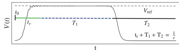
Figure 3: The HVCM is periodically activated with rise time  $t_r$  and pulse width  $T_1$  defined such that  $|V(t) - V_{\text{ref}}| < \frac{|V_{\text{ref}}|}{100}$  for all  $t \in [t_r, t_r + T_1]$ . The HVCM is then turned off for a length of time  $T_2$  such that the period  $T$  of one operation cycle is equal to  $t_r + T_1 + T_2 = \frac{1}{r}$ , resulting in  $r$  pulses per second.
