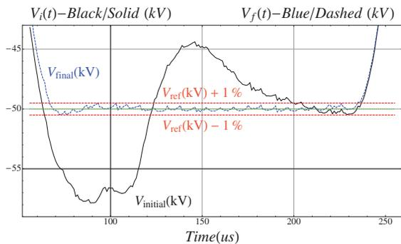
Figure 6: Using the averaging scheme and 8 edges per driving waveform the final output voltage was within 1% error after extremum seeking was completed.
