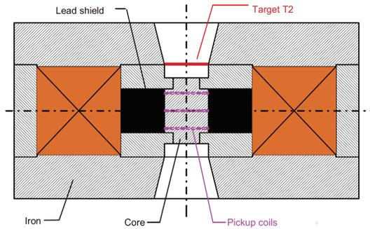
Figure 2: Schematic of the analyzing magnet horizontal section [5].
