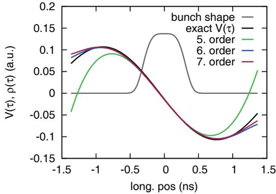
Figure 1: Beam induced voltage in the passive harmonic cavities from a quartic electron distribution. Comparison of the exact result with a Taylor-series expansion of the electron distribution up to different orders.
