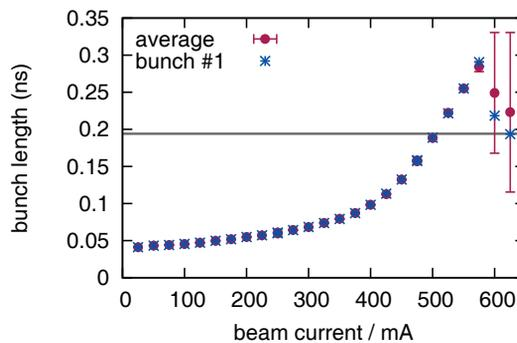
Figure 4: Bunch length under the influence of the HC. From the natural bunch length of 40ps, the beam induced voltages lengthens the bunches up to 190 ps for the nominal operation current of 500 mA, indicated by the gray line. The red points show the averaged values and its standard deviation over all bunches and the last 1000 turns before the current gets increased.
