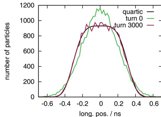
Figure 2: Initial Gaussian and final quartic charge distribution under the influence of the passive HC.
