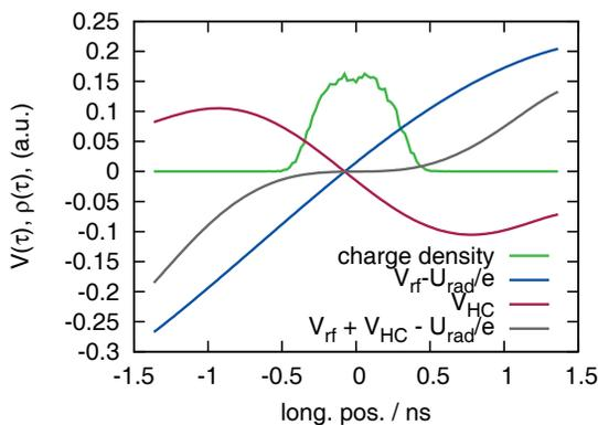
Figure 3: Rf-voltage, beam induced voltage and sum of the potential in comparison with a charge distribution snapshot from multibunch tracking.
