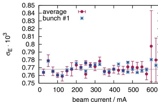
Figure 5: Energy spread development for increasing current: Every 50,000 turns the current is increased by 25 mA. The errorbars are the standard deviation of the value for all bunches and over 1000 turns.
