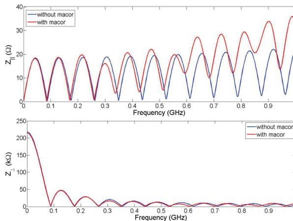
Figure 3: Longitudinal (top) and transverse (bottom) beam coupling impedance for striplines with and without Macor rings, simulated with CST PS.
