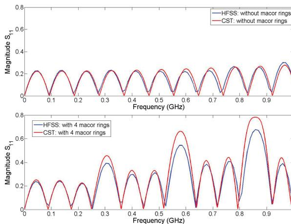
Figure 2: Magnitude of  $S_{11}$  predicted by HFSS and CST MS, for striplines without (top) and with (bottom) Macor rings.
