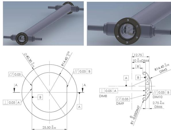
Figure 1: Prototype striplines and fabrication tolerances for the electrode supports and the electrodes.
