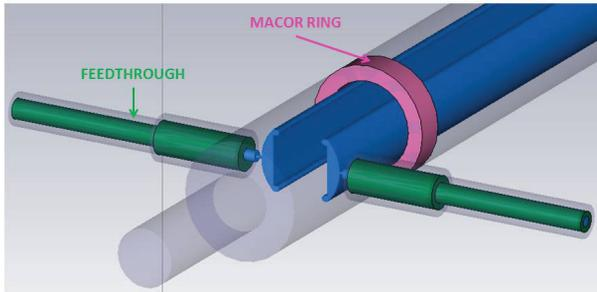
Figure 4: CST MS model used to optimize the electrode supports and the feedthroughs.
