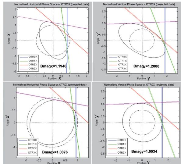
Figure 5: Top: initial normalised transverse phase space before beta matching. Bottom: normalised transverse phase space after 3 beta matching iterations. The dotted ellipse represents the designed (reference) phase space.
