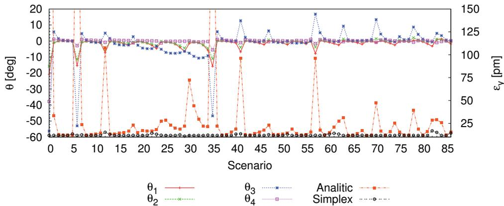
Figure 4: Coupling correction comparison of matrix response method and simplex method for various sets of coupling scenarios.
