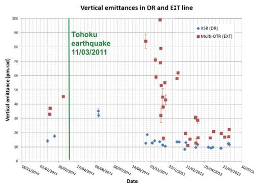
Figure 1: Summary of vertical emittance measurements at different dates in the damping ring and in the extraction line of ATF2 during 2011 and half 2012.
