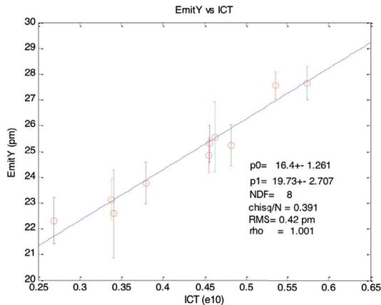
Figure 2: Vertical emittance as a function of the bunch charge (in units  $10^{10}$  particles per bunch) in the ATF2 EXT line.
