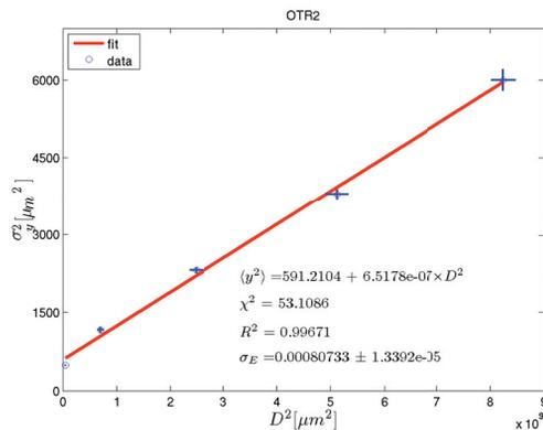
Figure 6: Energy spread measurements at OTR2.
