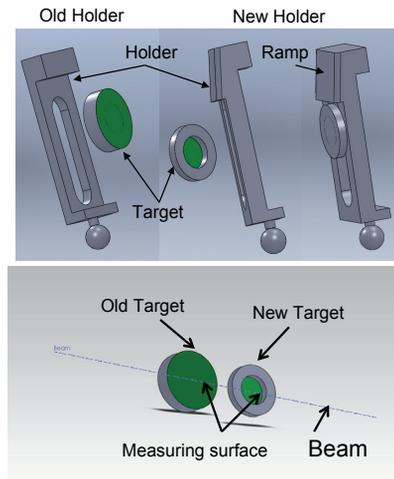
Figure 7: Comparison of old (left) and new (right) target holders.
