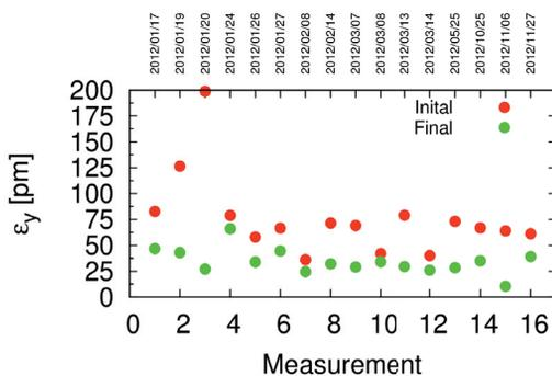
Figure 3: Vertical emittance measured before (initial) and after (final) coupling correction for various sets of measurements in 2012.
