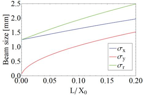
Figure 3: Beam size at absorber vs. spoiler length for EC1.
