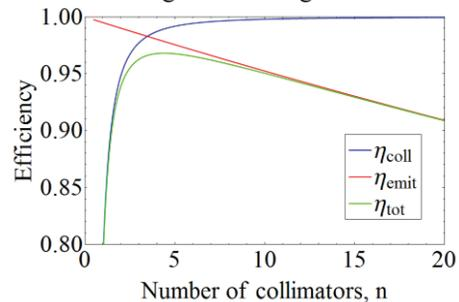
Figure 6: Collimation efficiency vs. the number of spoiler-absorber pairs in the BC system.
