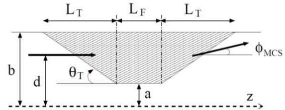
Figure 2: Longitudinal sketch of a spoiler or absorber.
