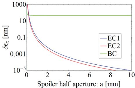
Figure 4: Emittance growth vs. spoiler half aperture for  $1\sigma_\beta$  beam jitter.
