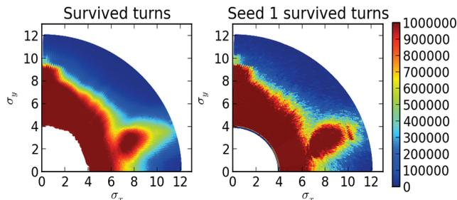
Figure 1: Survival plot in the transverse action plane for  $1.2 \cdot 10^6$  particles tracked for  $10^6$  turns in the LHC. A smoothing over 10 amplitudes (right) or over 60 seeds (left) highlights the lifetime figures of single particles as a function of the initial transverse amplitudes.
