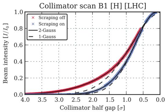
Figure 2: Collimator scans in the LHC after injection of beam with and without tail scraping in the SPS are shown. Both a double and a single Gaussian function have been fitted to the data. For the scraped beam the tails are much smaller and the profile is very close to a Gaussian.
