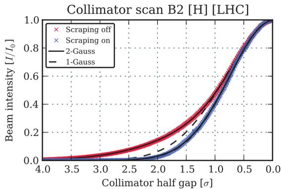
Figure 3: Collimator scans for beam 2 with and without scraping are shown. Both a single Gaussian and a double Gaussian have been plotted. For the beam which has been scraped the two lines are identical.
