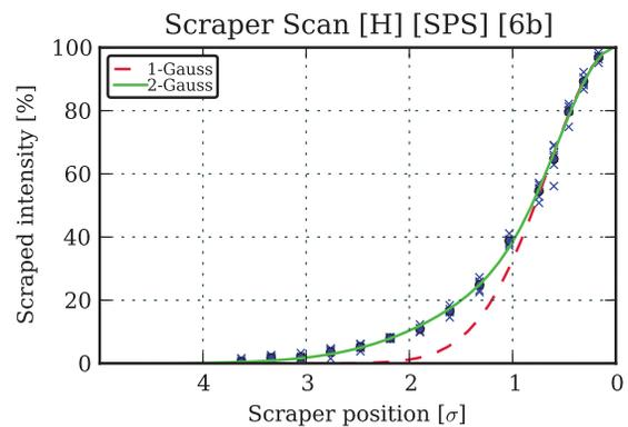
Figure 4: Beam scan was done in the SPS using a beam of 6 nominal bunches for injection loss measurements. The double Gaussian fit indicates that there are large tails.
