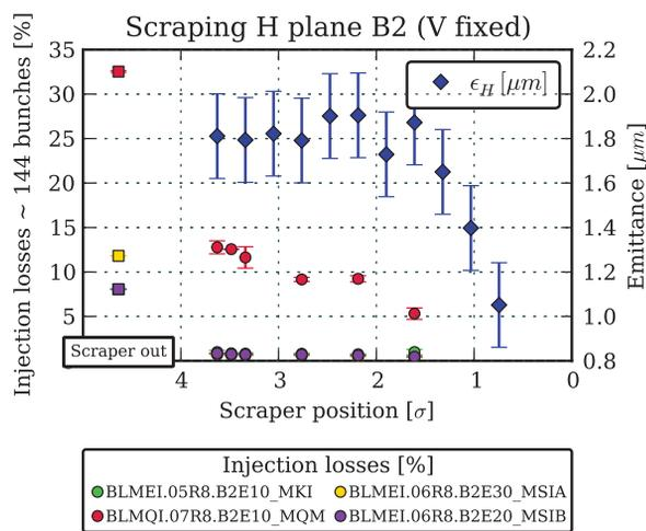
Figure 5: Beam losses at injection for varying scrapper depths are shown for beam 1. The losses are scaled to 144 bunches and taken with respect to the LHC dump thresholds. If the beam is not scraped the losses are above 50 % of dump thresholds. Scraping reduce the losses to an acceptable level already at 3  $\sigma$  while the emittance is not reduced until around 2  $\sigma$ .
