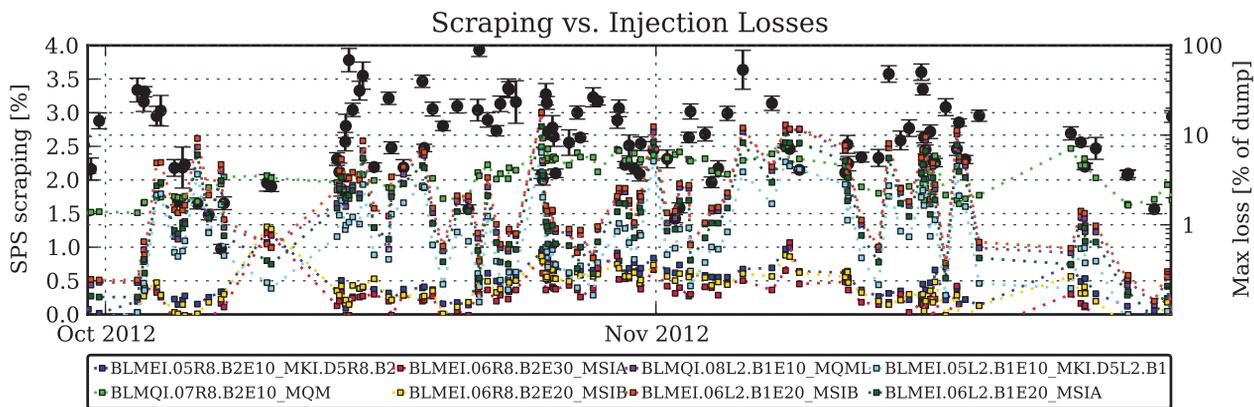
Figure 7: The amount scraped for LHC fills is given in black. Normally 2-4 % of the beam is scraped to remove tails. The beam losses are given for a number of BLMs in the injection region.
