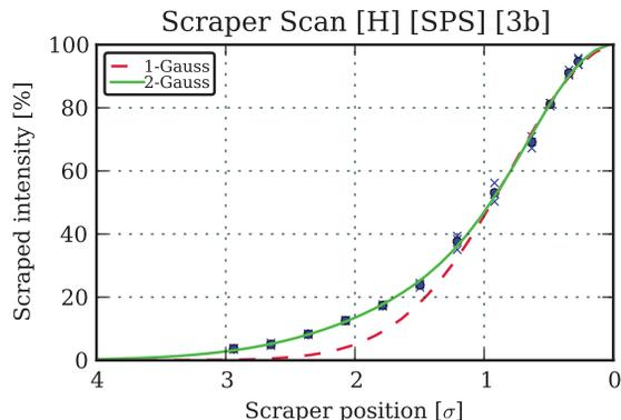
Figure 1: A beam scan done by the scraper in the SPS as a reference for scans in the LHC after injection. The measurements are fitted by a single and a double Gaussian. Because of the large tails the double Gaussian function gives the best approximation.
