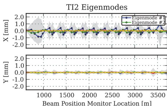
Figure 3: The plot shows trajectory variations after the SPS optics change. The variations have approximately the same size as before, but the pattern is different.
