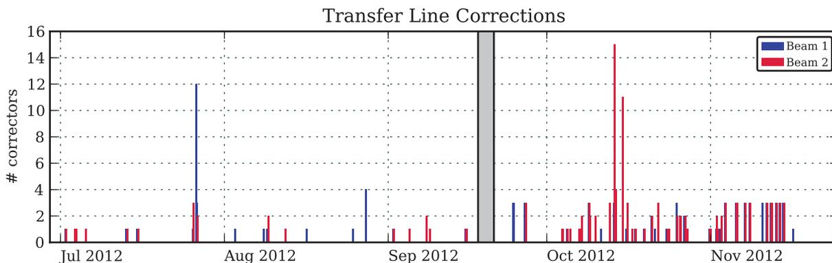
Figure 1: Frequency of transfer line corrections are shown for a period in summer with normal optics and for a period after the SPS optics change during the technical stop (shown in grey). The correction frequency dramatically increased from 1-2 times per week to almost daily in the second period.
