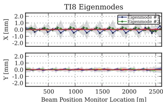
Figure 4: Trajectory variations for TI 8 before the technical stop are shown. In the horizontal plane there are large variations coming from two independent sources.
