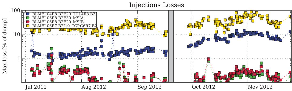
Figure 7: Maximum beam loss at injection per fill for selected beam loss monitors. After the last technical stop (shown in grey) an increase in the losses at the TDI and downstream at the TCP was observed. This loss signature indicates that the losses are longitudinal. Losses from the transverse plane (given by the BLMs at the MSI) remained low.
