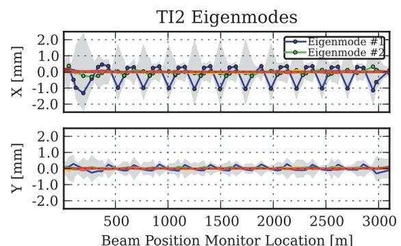
Figure 2: The observed variations for a period before the last technical stop is shown in grey. The variations are around 3 mm peak-to-peak in the horizontal plane. The MIA eigenmodes are given in the plot scaled by their eigenvalues. Only the two largest ones give a significant contribution indicating that there are two sources of variation. In the vertical plane the variations are small.
