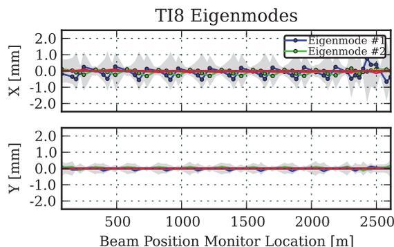
Figure 5: The plot shows the observed (grey) and calculated trajectory variations in TI 8 after the technical stop.
