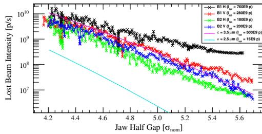
Figure 5: Beam tail population calculated from the BLM signals at the TCPs, during the scan on May 15<sup>th</sup>, 2012. Expected populations for two emittance values are given.
