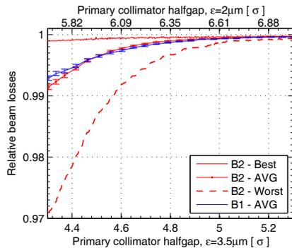
Figure 3: Average B1 and B2 losses during the ramp versus TCP half gap, for  $\epsilon = 3.5\mu\text{m}$  (bottom axis) and  $\epsilon = 2.0\mu\text{m}$  (top). Best and worst loss cases for B2 are also given. Errors on the average are estimated as the R.M.S. of the measured points divided by  $\sqrt{n_{\text{fill}}}$  ( $n_{\text{fill}} = 110$ ).
