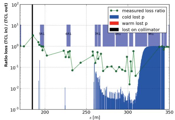
Figure 7: Ratio of the simulated losses for the case “TCL in” ( $10\sigma$ , Fig. 4 top) over the case “TCL out” ( $60\sigma$ , Fig. 4 bottom), for the range of  $s$  for which the SixTrack simulations are meaningful. The black line represents the TCL.5R1.B1. The green curve represents the ratio for the measurements in the LHC, as shown in Fig. 2.
