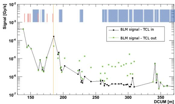
Figure 1: BLM signals on the right side of IP1 ( $s = 0$  m) for “TCL in” (black) and “out” (green) with a luminosity of  $\simeq 4 \cdot 10^{33} \text{ cm}^{-2} \cdot \text{s}^{-1}$ . Layout elements are illustrated by red and blue boxes. The TCL sits at  $s=184$  m (orange line).
