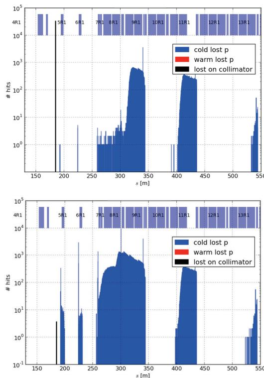
Figure 4: Losses simulated by SixTrack for the losses downstream TCL.5R1.B1 (at 184 m). Top: TCL set at  $10\sigma$ , bottom:  $60\sigma$ . The initial distribution had  $1.77 \cdot 10^6$  particles, corresponding to  $10^7$  p-p interactions.
