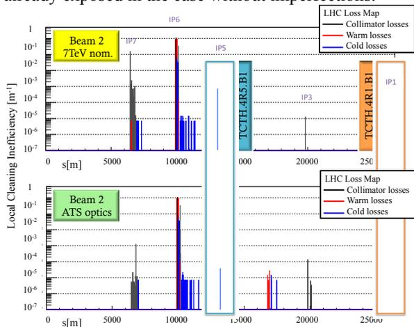
Figure 4: Local cleaning inefficiency loss maps for Beam 2 applying errors. It has to be noted that TCT at Point 5 set at 7.3  $\sigma$  shields the Point 1 TCT.
