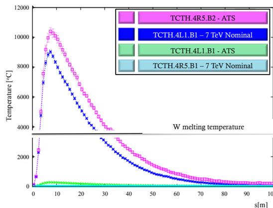
Figure 5: Temperature peaks in the tungsten TCT inserts. In the figure the most loaded jaw per TCT is shown. In case of errors, 2 critical TCT locations are put in evidence for the different optics. In particular for the LHC upgrade the Beam 2 TCT location at Point 5 is resulting the most exposed one.
