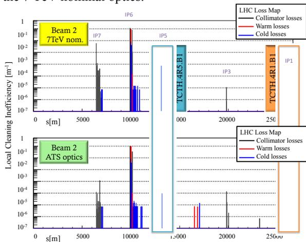
Figure 3: Local cleaning inefficiency loss maps comparison for Beam 2, perfect machine. The Point 5 peak (blue area) has to be noted. Located just downstream IP6 and with phase advance close to 90°, the TCT is already exposed in the case without imperfections.
