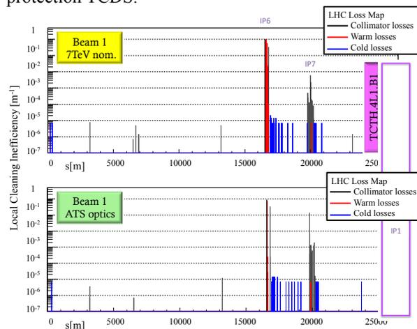
Figure 2: Simulated loss maps around the LHC ring, when errors are introduced. The highest contribution to the TCT peak at Point 1 is due to the retraction of the 4 critical collimators at Point 7. It has to be pointed out that in case of ATS optics a favorable phase advance between the kickers location and the horizontal primary collimator plays a major role to protect the TCT (i.e. TCP.C6L7.B1 at about  $77^\circ$  phase advance).
