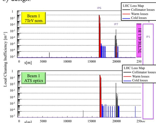
Figure 1: Local cleaning inefficiency loss maps for ATS and 7TeV nominal optics, for perfect machine. Results are normalized to the maximum of losses at the extraction protection TCDS.
