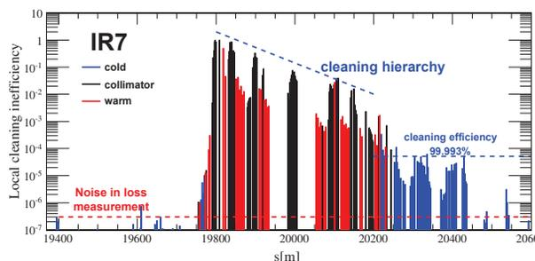
Figure 5: Distribution of the losses in the betatron cleaning insertion (IR7) while exciting Beam 1 in the horizontal plane.
