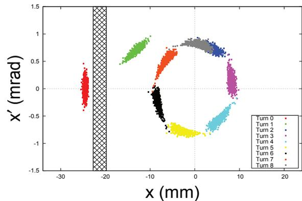
Figure 2: The injection simulation for a multiparticle beam in horizontal phase space at injection point. The first eight turns of particles tracking are shown. The black cross lines represent the septum wall with a thickness of 3 mm.
