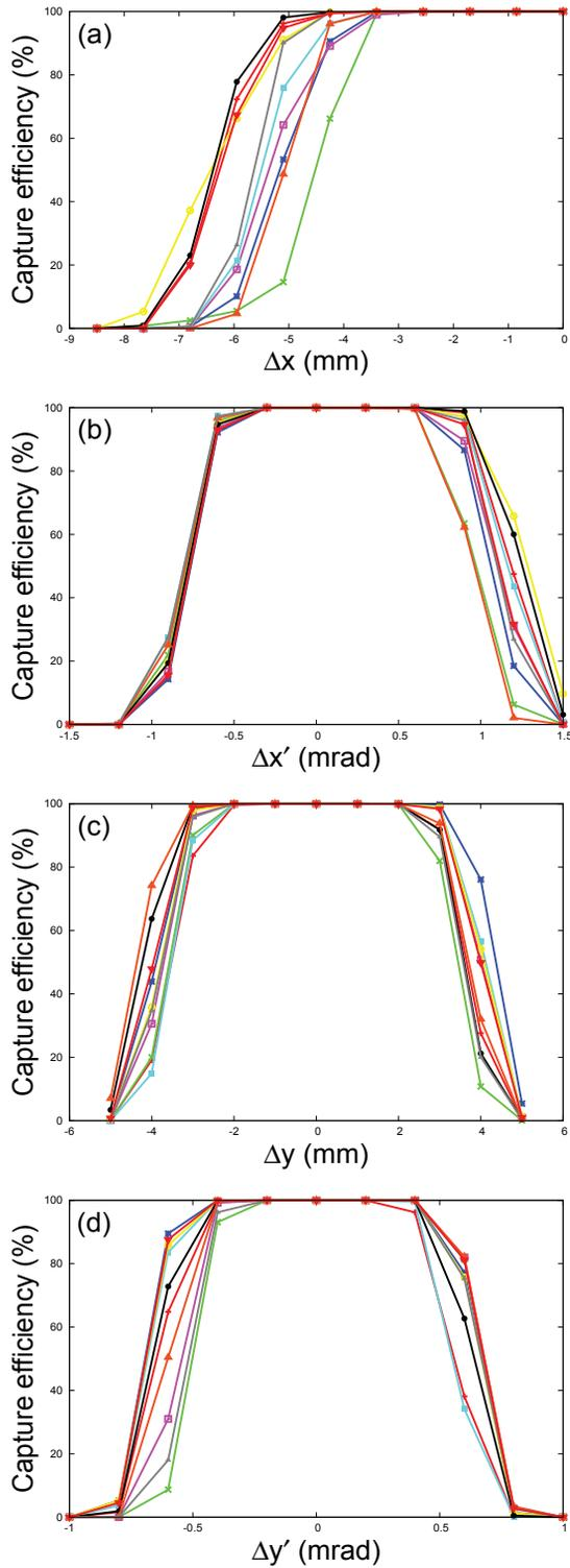
Figure 3: The capture efficiency vs. the deviation of launching condition for an injected beam on (a)  $x$ -, (b)  $x'$ -, (c)  $y$ - and (d)  $y'$ -direction. There are 10 random lattice models used for injection simulations.
