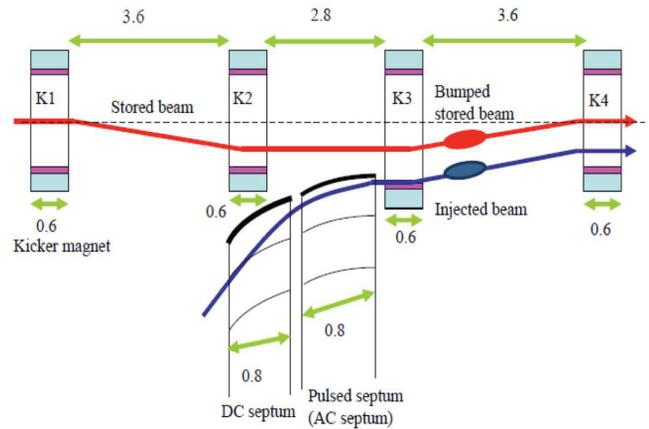
Figure 1: The layout of off-axis injection for TPS storage ring, in the units of meters.
