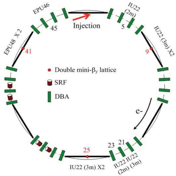
Figure 4: The particle loss distributions in TPS storage ring are shown in the upper plot. The locations of straight sections which contain IDs are marked as light yellow columns. Lower plot is the corresponding layout of TPS storage ring with port numbers which contain double-mini- $\beta_y$  and IDs.
