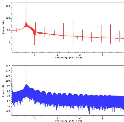
Figure 3: (top) Synthetic spectra generated by harmonic modulation of a spatially uniform plasma dielectric at the revolution frequency. (bottom) Synthetic spectra generated by translating cloud densities.
