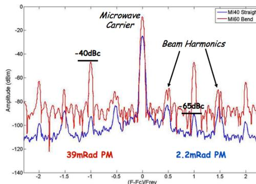
Figure 1: Spectral data showing side bands induced by electron cloud plasmas in the Main Injector for two different magnetic field configurations. The height of the first side band is nominally proportional to the average cloud density in the linear approximation. Reproduced from [3].
