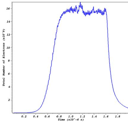
Figure 2: Total number of electrons as a function of time, showing electron cloud buildup and dissipation. Kinetic simulation results are used in our plasma dielectric simulations to set the dielectric strength.
