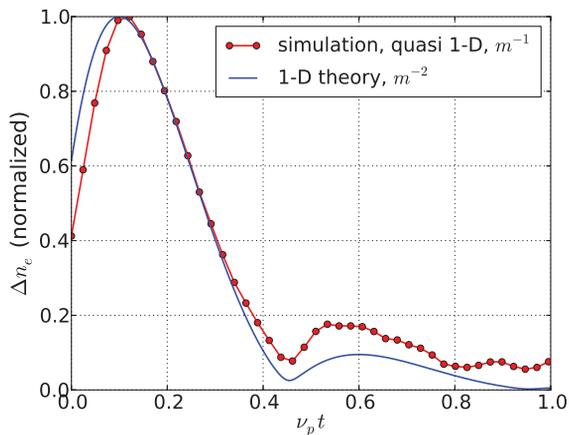
Figure 3: Peak magnitude of electron bunch charge density modulation as a function of its propagation time in the kicker.
