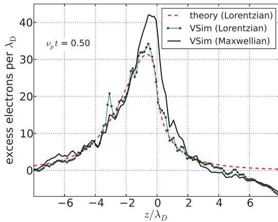
Figure 1: VSIM  $\delta f$  PIC computation of longitudinal on-axis electron density perturbation near a  $\text{Au}^{+79}$  ion with a non-zero longitudinal velocity in an anisotropic plasma.
