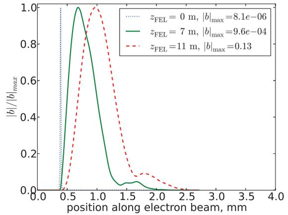
Figure 2: Normalized bunching magnitude, at  $\lambda_{\text{FEL}}$ , along the electron beam at different positions in the FEL. The bunching magnitude increased from  $|b|_{\text{min}} = 8.1 \times 10^{-6}$  to  $|b|_{\text{max}} = 0.13$ .
