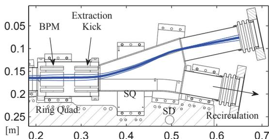
Figure 2: Centroid tracking for a matched 23 mA beam, in more recent design.
