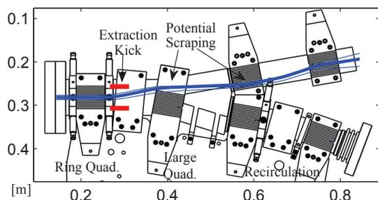
Figure 1: Centroid tracking for a matched 23 mA beam, in original extraction design. The best-possible centroid motion in this design was deemed too intractable for use with higher current.
