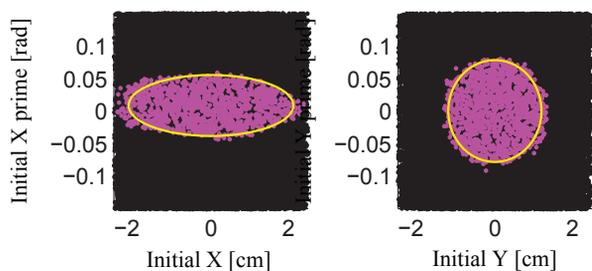
Figure 3: "Zero-current" acceptance of recirculation. X,Y axes correspond to particle initial condition. Black particles are lost on the absorbing boundary, magenta particles survive through one turn (11.52 m).
