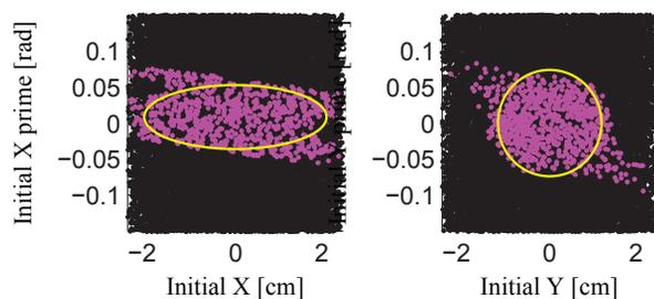
Figure 4: "Zero-current" acceptance for extraction. See Fig. 3. Particles propagate 64 cm through extraction.
