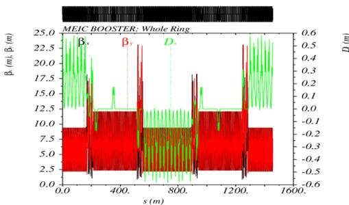
Figure 3: This is a MAD-X plot of the lattice functions of the large booster.
