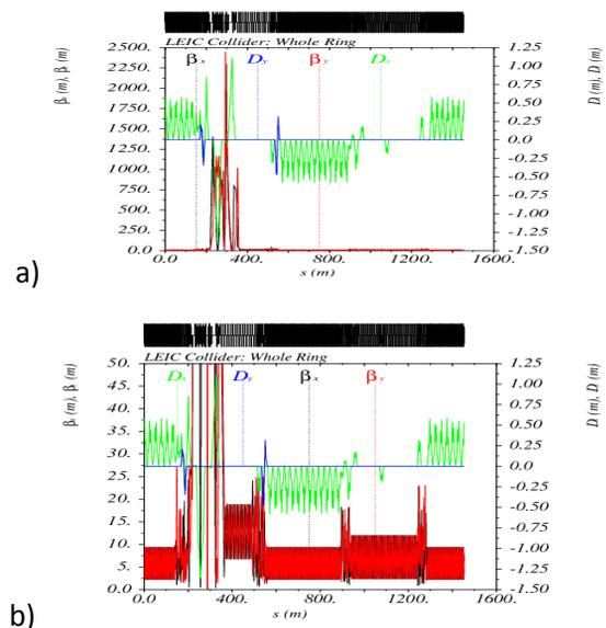
Figure 6: a) The complete lattice functions of the LEIC ring, the large beta functions are a result of the matching for the interaction region. b) This is a truncated version that allows a closer inspection of the lattice functions of the rest of the ring.
