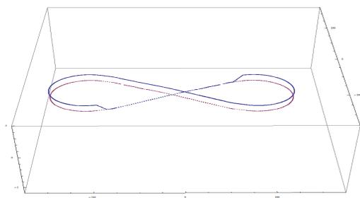
Figure 4: Physical arrangement of the LEIC above the plane of the electron ring, the vertical axis uses a different scale from the two horizontal axes for better visibility.
