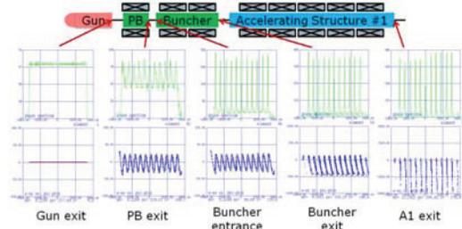
Figure 4: The process of beam bunching.
