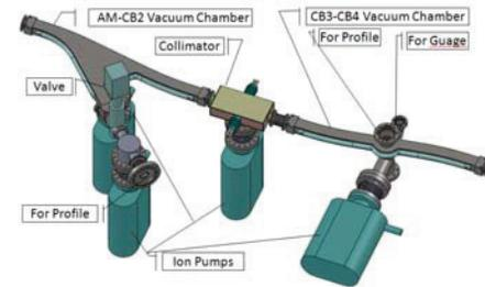
Figure 3: 3D model of chicane vacuum system.
