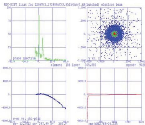
Figure 5: Beam performance at the bunching system exit.
