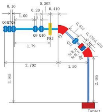
Figure 6: Layout of the transport line.
