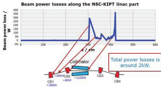
Figure 2: Layout and beam losses distribution in KIPT linac chicane and accelerating system.
