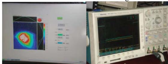
Figure 7: Electron beam profile and pulse at the exit of the first accelerating section.
