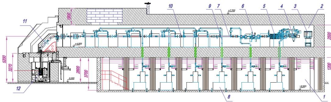
Figure 1: Layout of the accelerator and subcritical assembly systems: 1 – klystron gallery, 2 – accelerator tunnel, 3 – electron gun power supply, 4 – injector part of the accelerator, 5 – the first accelerating section, 6 – chicane, 7 – accelerating section, 8 – klystron, 9 – wave guide, 10 – quadrupole triplet, 11 - electron beam transportation channel, 12 – subcritical assembly.
