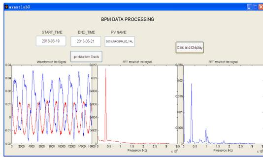
Figure 4: BPM data processing using MATLAB.
