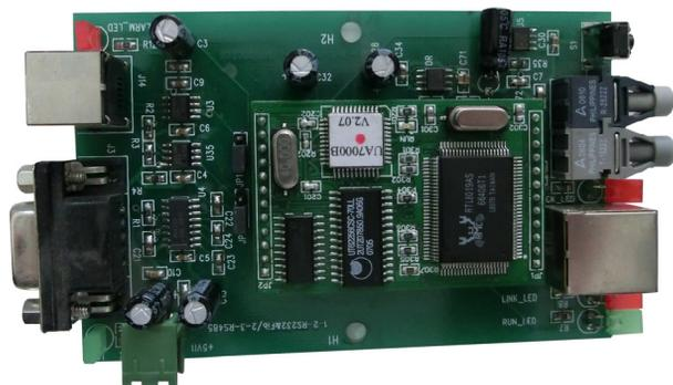
Figure 2: Protocol-and-signal converter.
