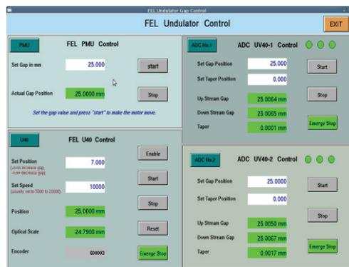
Figure 3: Operator interface for undulator gap adjustment.
