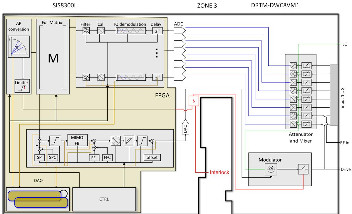
Figure 3: Hardware and firmware block diagram of the LLRF controls
