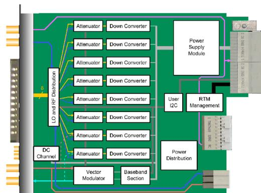
Figure 1: Block diagram of the DRTM-DWC8VM1 board.
