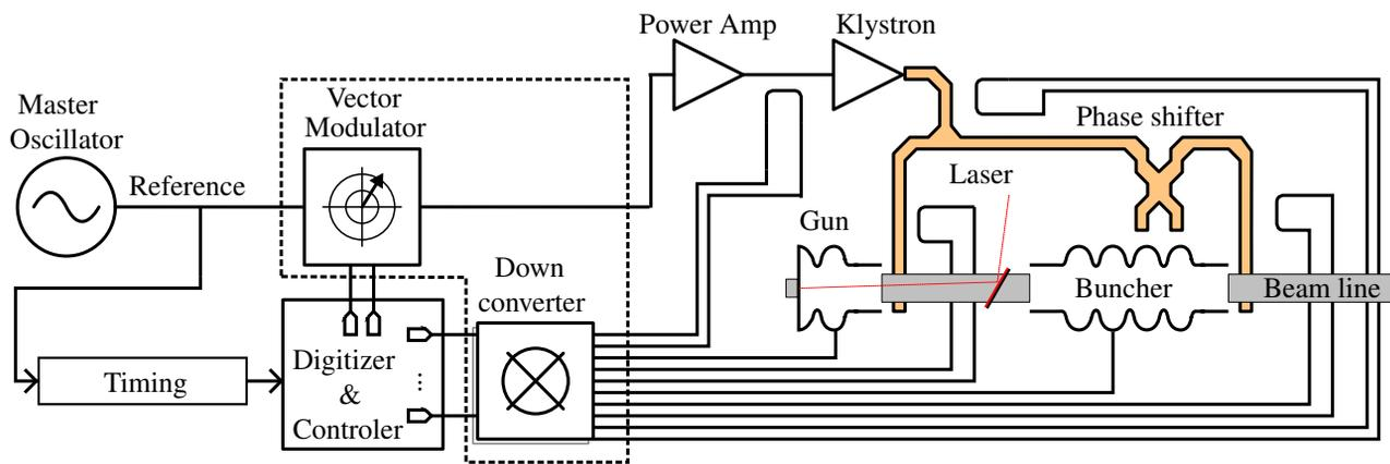
Figure 2: REGAE low level and high power RF systems block diagram
