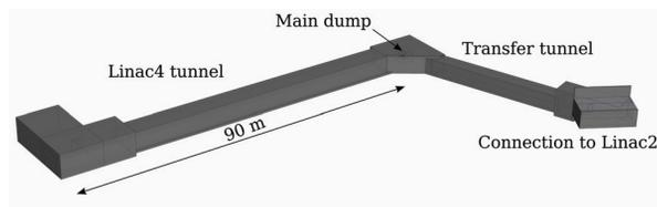
Figure 1: FLUKA geometry of the tunnel enclosure.
