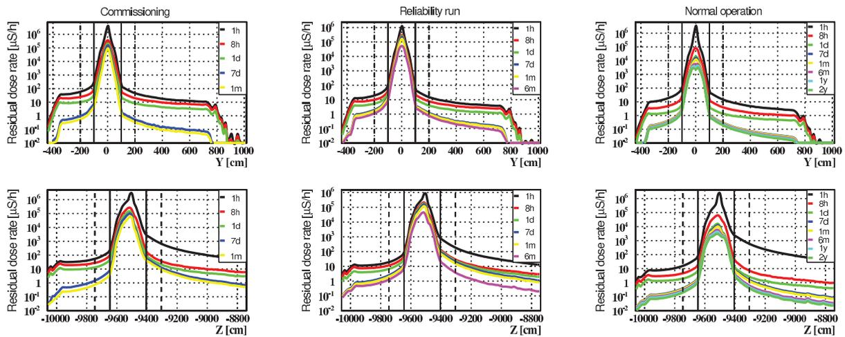
Figure 3: Ambient dose equivalent rates after several cooling times on an imaginary plane at center of the dump perpendicular (top) and along the beam direction (bottom) for three operation phases. Full vertical lines indicates the shielding boundary and dashed lines mark a 1 m distance from the shielding.
