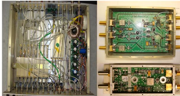
Figure 5: The RF Support Chassis (left) with Up Convert (right-up) and Down Mixer Modules (right-bottom).
