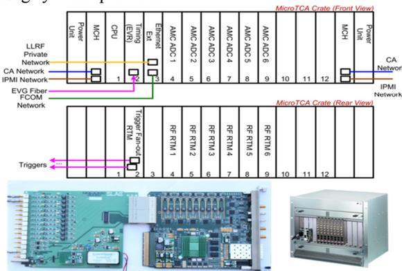
Figure 6: 12-slot MicroTCA Crate for LCLS-II Injector LLRF and AMC-ADC Board-Struck SIS8300 with SLAC RTM.
