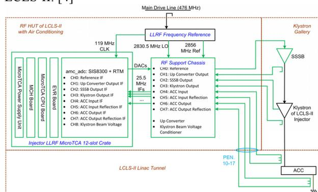
Figure 4: Architecture of a typical Klystron Station Control.
