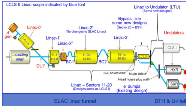
Figure 1: LCLS-II Structure Layout.
