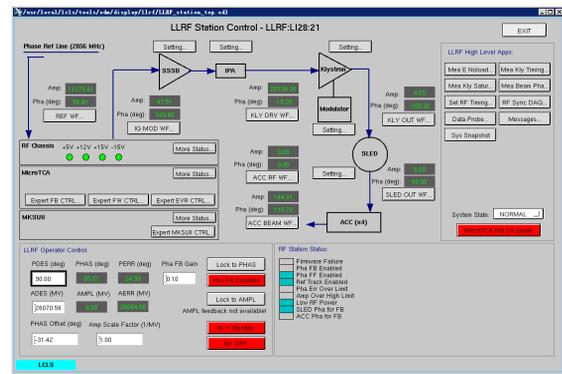
Figure 9: Users' Panel for RF Station Control.
