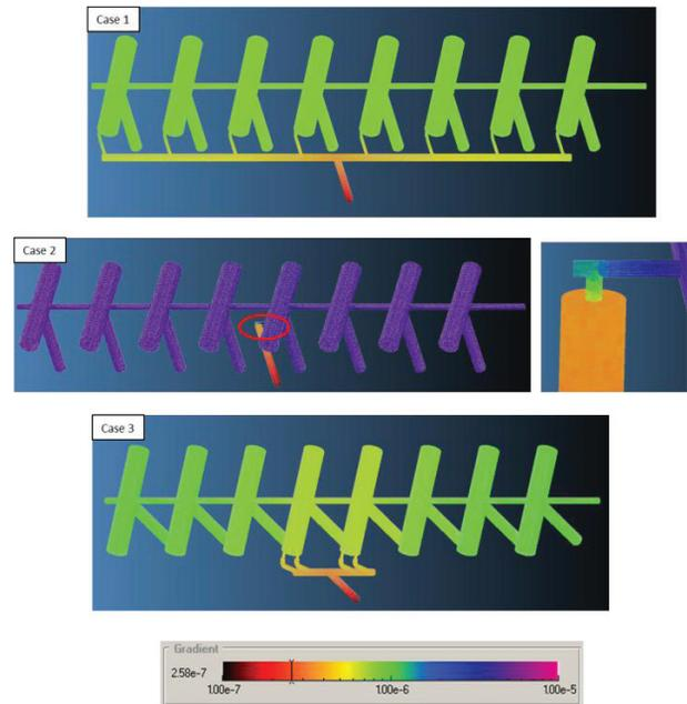
Figure 4: results of the pressure calculations for the three studied configuration: vacuum manifold connected to all the cavities (case 1), pumping through the pick-up port of the central cavity (case 2), vacuum manifold connected to two central cavities (case 3).
