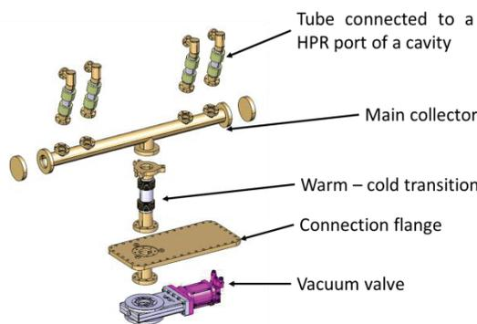
Figure 6: The vacuum manifold.
