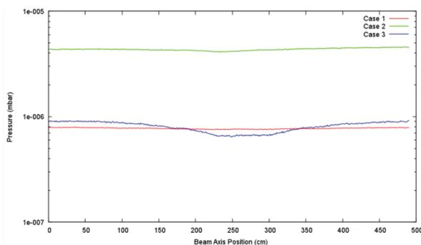
Figure 5: pressure profile along the beam axis depending on the pumping configuration: vacuum manifold connected to all the cavities (case 1), pumping through the pick-up port of the central cavity (case 2), vacuum manifold connected to two central cavities (case 3).
