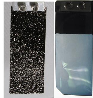
Figure 1: Left: HBC-foil at KEK, Right: Diamond foil at SNS.
