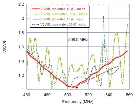
Figure 3: Broadband performance of the tap-water and pure water (measured and calculated value).
