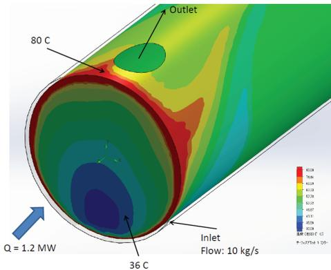
Figure 8: Temperature distribution in the load with dummy heat load (1.2 MW).
