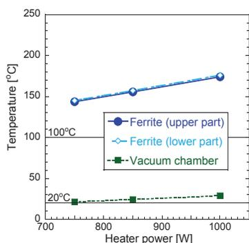
Figure 3: Heater power dependence of the ferrites and the vacuum chamber temperatures.
