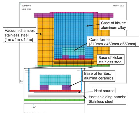
Figure 1: Calculation model for the thermal analysis.
