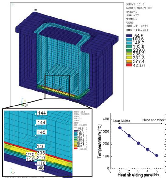
Figure 2: Typical temperature distribution of a kicker magnet and vacuum chamber. This is the case of heater power of 850 W.
