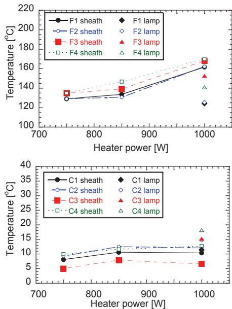
Figure 5: Measured temperatures of each point. F1-4 and C1-4 represent the thermometric points in Fig. 4.
