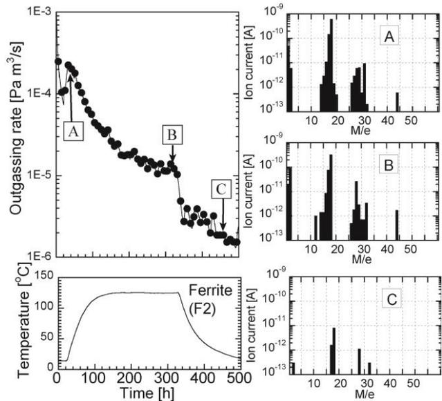
Figure 7: Results of the outgassing reduction by using the circular lamp heater. The applied heater power is 1000 W.
