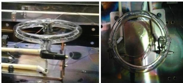
Figure 6: A circular halogen lamp heater. The main gas (Ar) is filled in the circular glass tube.
