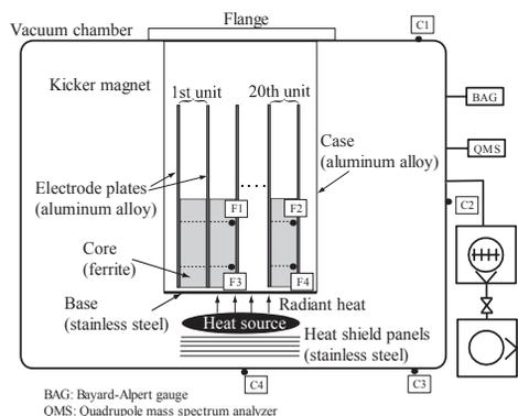
Figure 4: Concept of experimental setup. F1-4 and C1-4 represent the thermometric points.
