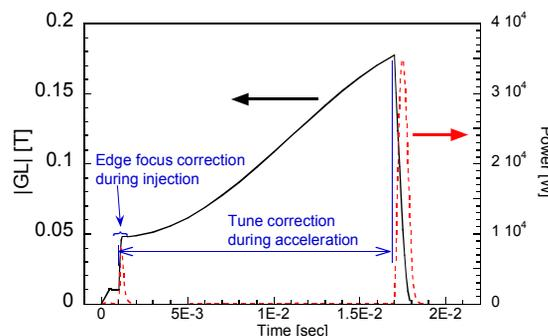
Figure 1: Black curb: time response of the absolute magnetic field of the quadrupole corrector. Red dotted curb: corresponding power, which is generated in a titanium duct by the eddy current.
