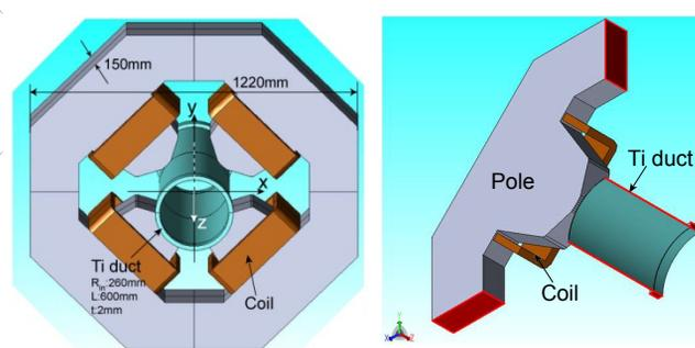
Figure 2: Full and 1/8 model for the calculation of eddy current effects. The actual calculation was performed by the 1/8 model.
