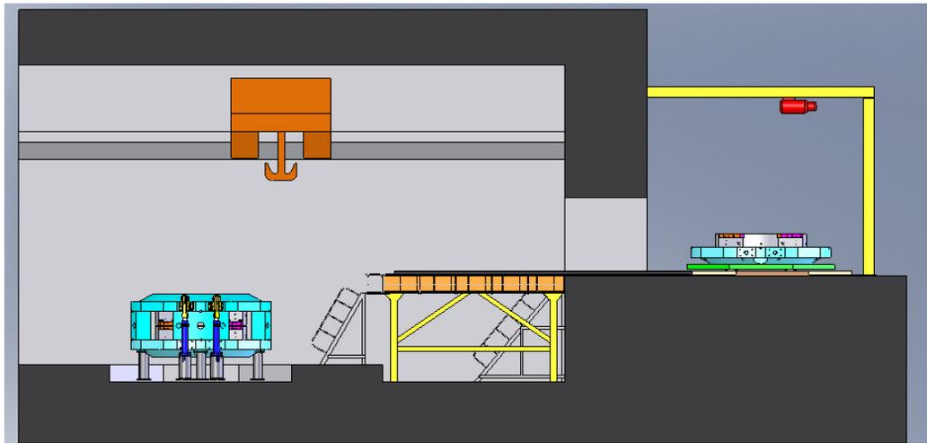
Figure 3: The unloading position and the mounting position of the main magnet.
