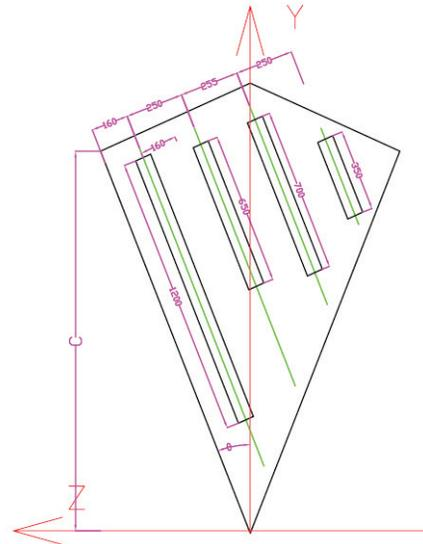
Figure 3: The layout of cryopanel, spacer and shield.
