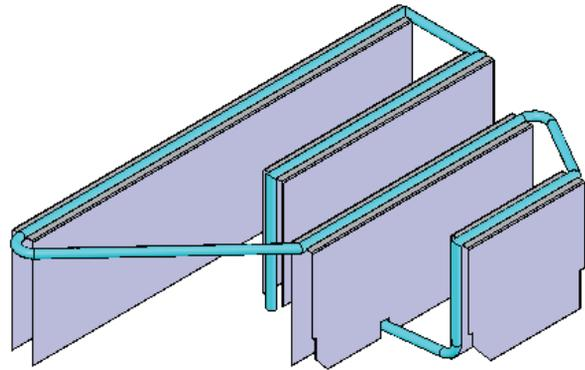
Figure 2: Cryopanel in shield.
