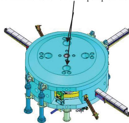
Figure 1: Two  $\Phi 500\text{mm}$  holes for external pump on the top yoke.
