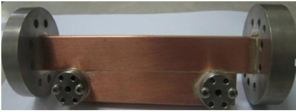
Figure 6: Prototype of the X-band waveguide directional coupler.
