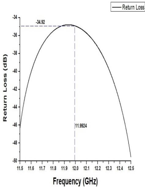
Figure 3: Frequency response of the Return loss.
