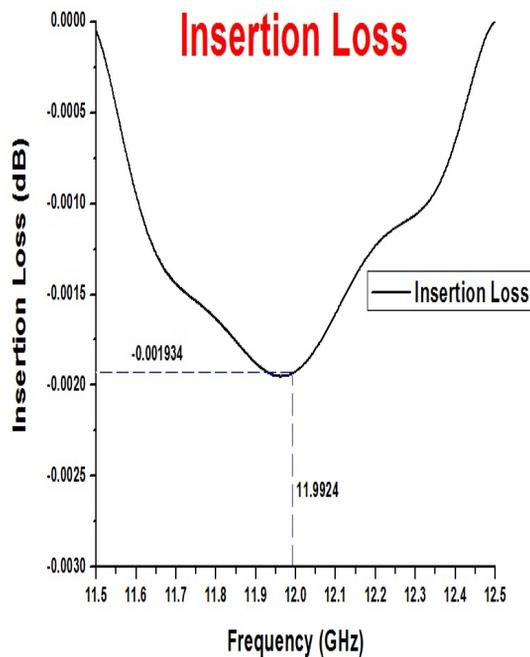
Figure 4: Frequency response of the Insertion Loss.
