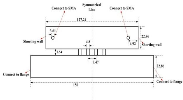
Figure 1: Structure of the X-band waveguide directional coupler (Looking down), Unit: mm.
