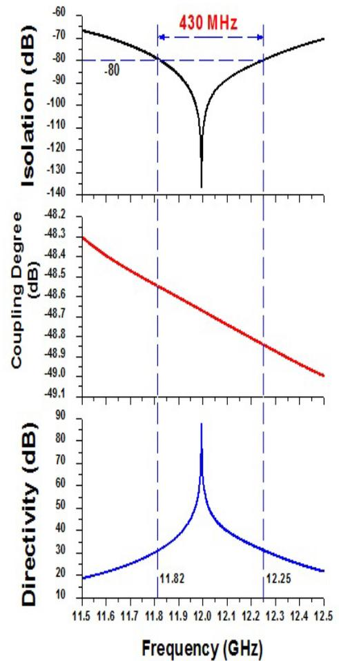
Figure 5: Frequency response of the Directivity, Coupling Degree and Isolation.
